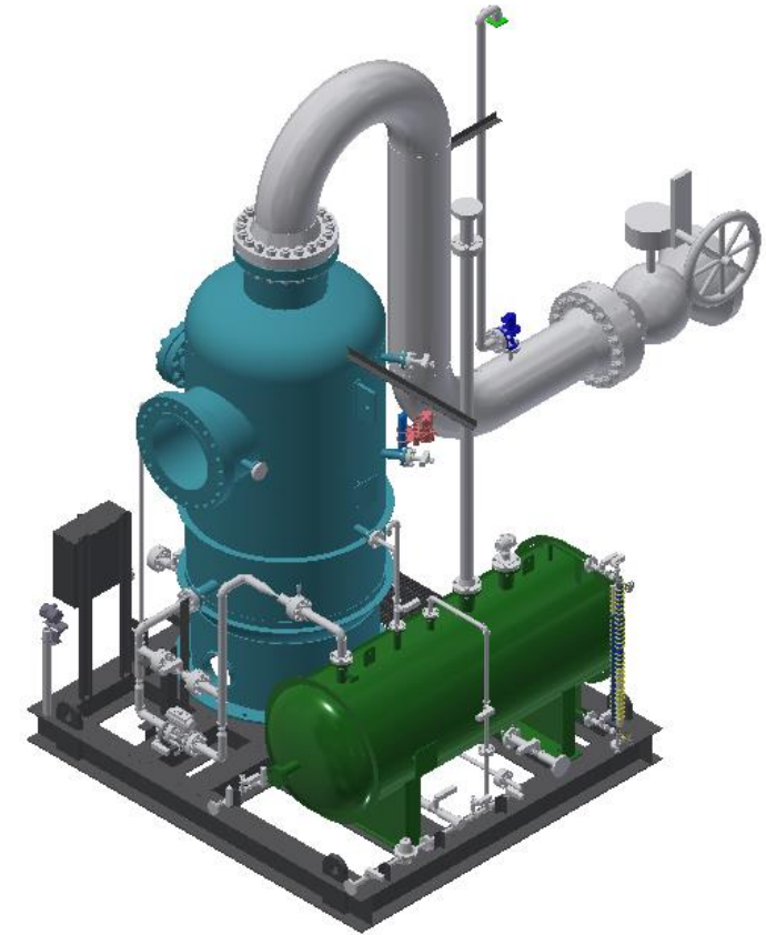
Assembled Drain Tank & Cyclone Scrubber
